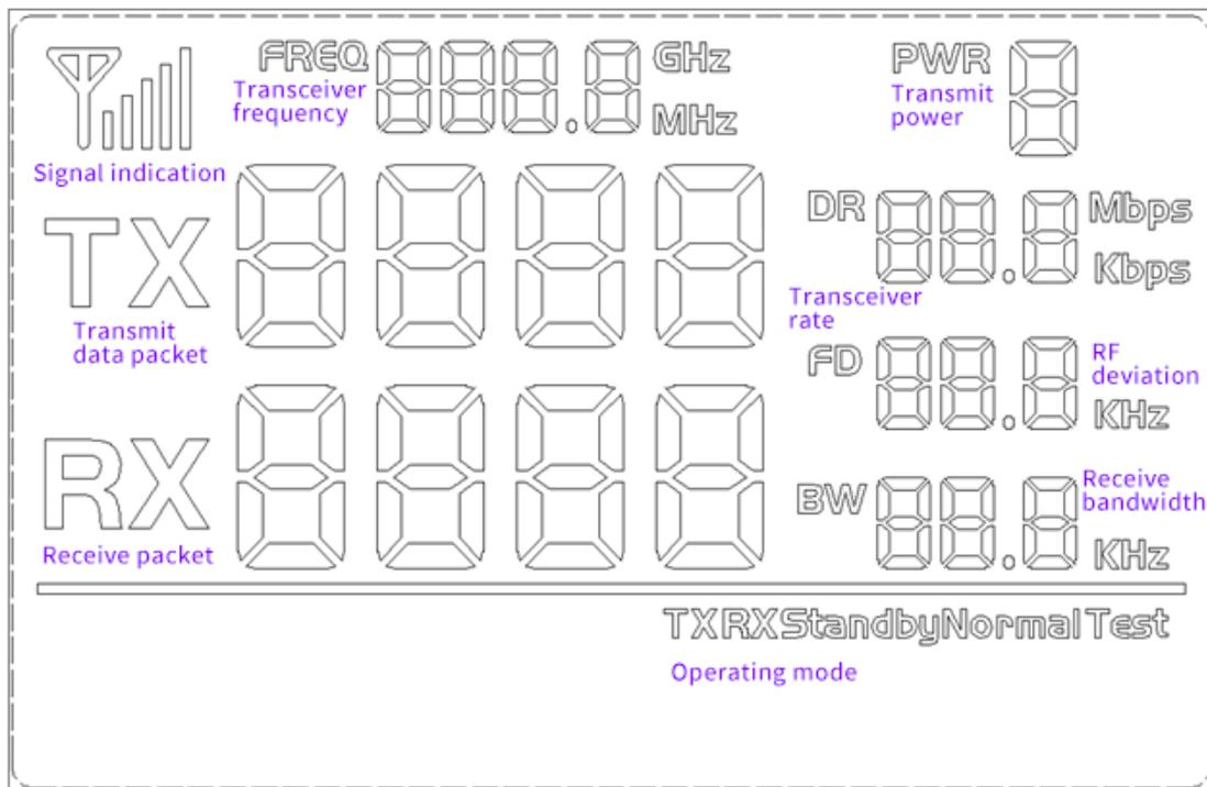
Users can set the parameters of the RF module such as working mode /frequency / transmitter power / transmission data rate through the buttons, and measure the wireless communication distance.
